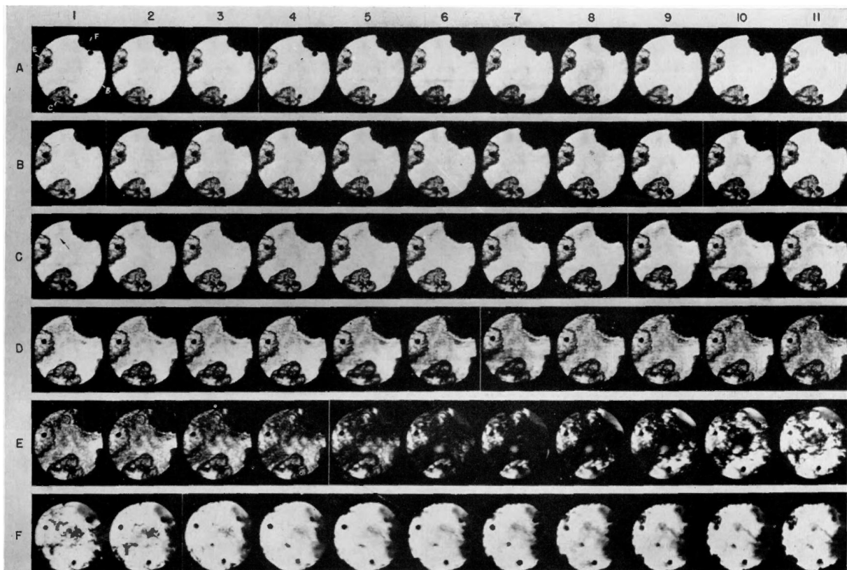
FIGURE 11.—High-speed motion picture of combustion of M-4 reference fuel showing extensive homogeneous autoignition followed by heavy knock.
